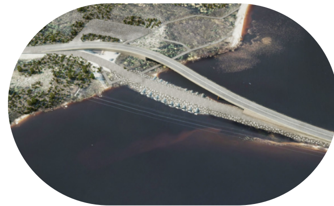
RENDERING OF THE NEW BRIDGE AND THE ACCESS ROAD WITH CULVERTS
